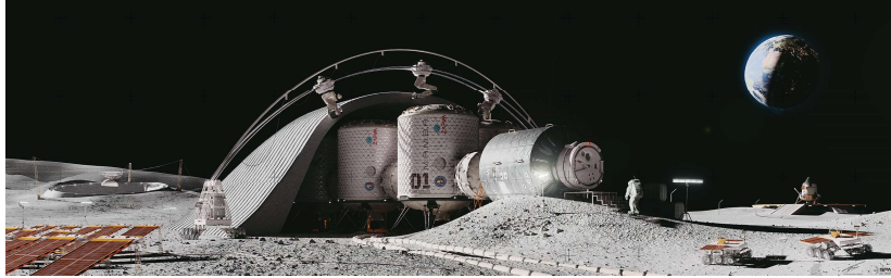
Figure 1: Rendering of six MaMBA modules and an airlock on the Moon covered artificial cave.
